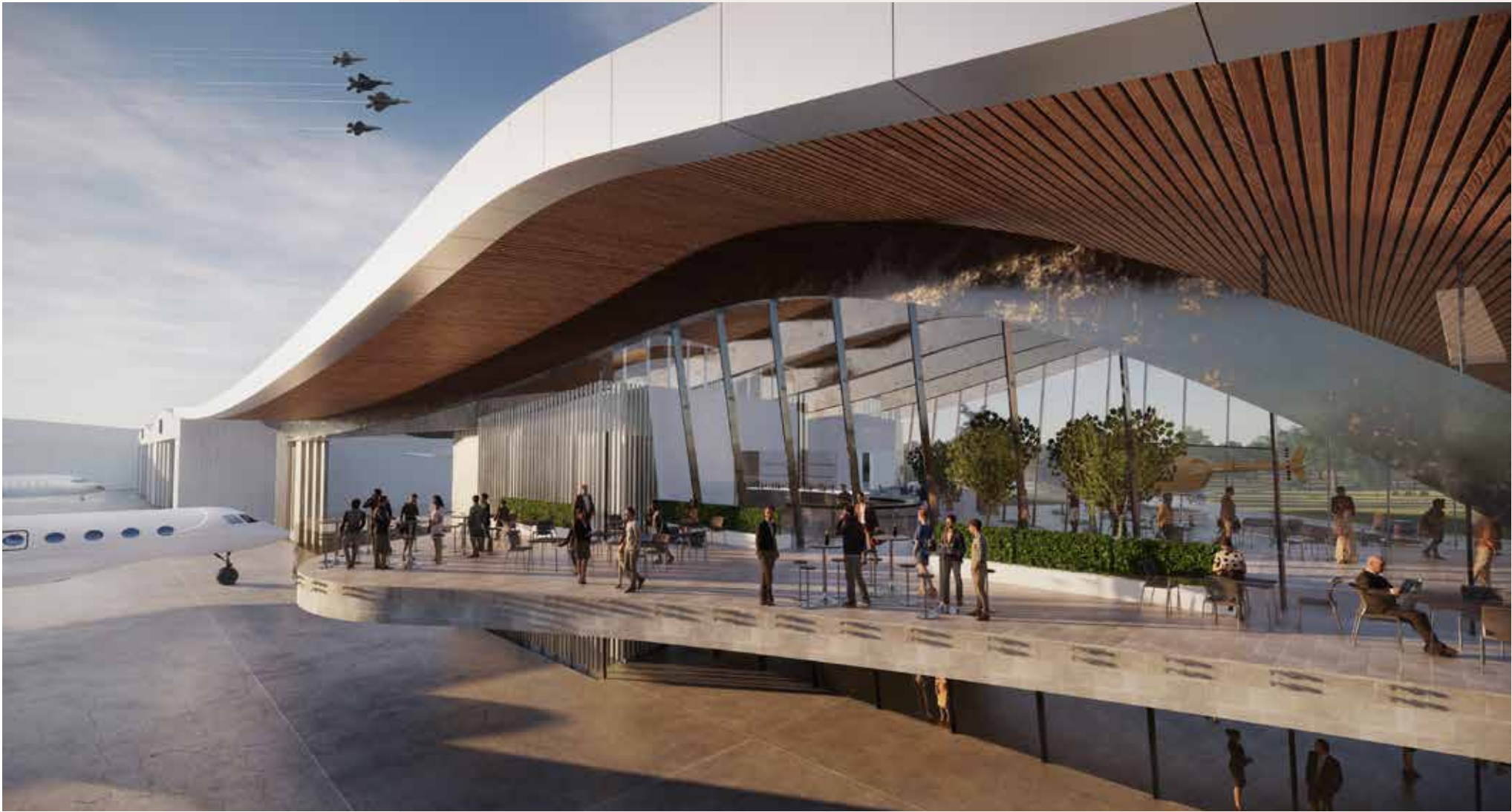
Solar protection for most of the day is provided by the oversailing roof and internal blinds for low angle sun.
