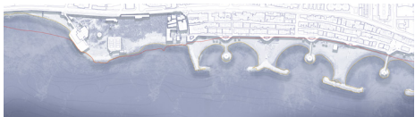
Current coastline with beach extension together with the use of breakwaters to reduce erosion and avoid flooding after 1980's
